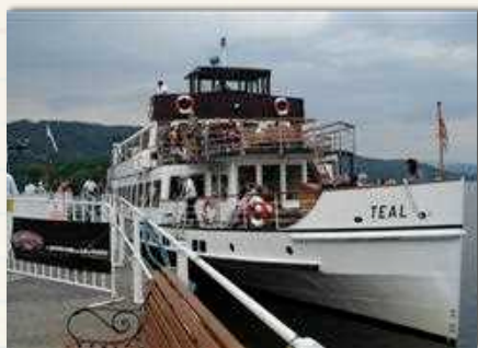
MV TEAL on Lake Windermere. Built by Vickers of Barrow in 1936. B2X 6 cylinder diesel engines with a crew of 7. 533 passengers.
