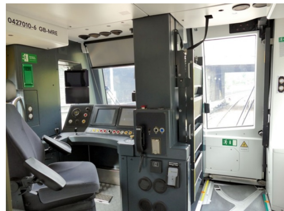
[Driver's cab- controls on left, emergency exit door on right with collapsible detrain ladder stored vertically on left of door]
