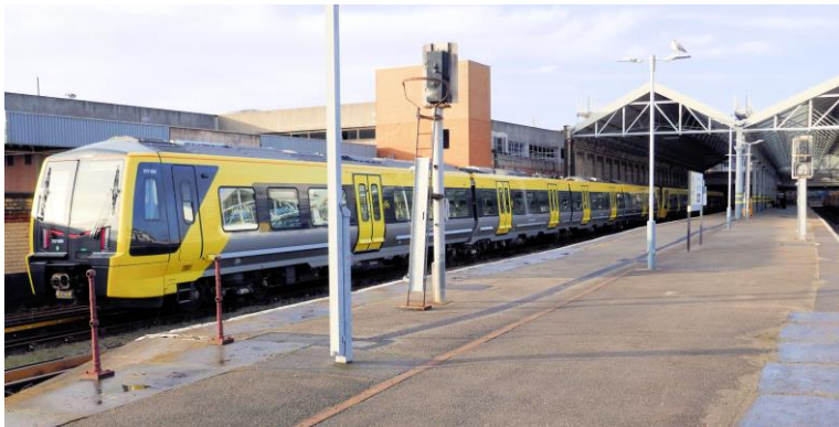
The pictures show Liverpool-bound platforms 1, 2 and 3 at Southport station, with a double-unit Class 777 in the holding siding next to the platform 1 track (left side of left pic). The platform 1 signal is just about in line with the driver's cab. Note the signal for platform 2 (right side of left pic) is much less further out on its platform. The signal on platform 3 is level with that on platform 2 (right pic), just before the points.
