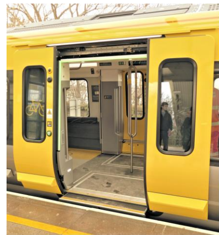
Door-operating buttons and platform-flush step
