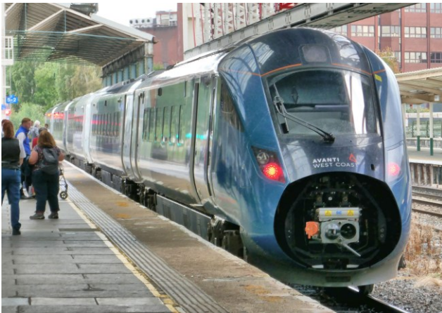
Evero unit with nose cowl removed to allow connection to a second unit
