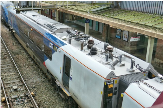
Lowered (inactive) pantograph at Chester station. (It is raised to access power from an overhead electric line)
